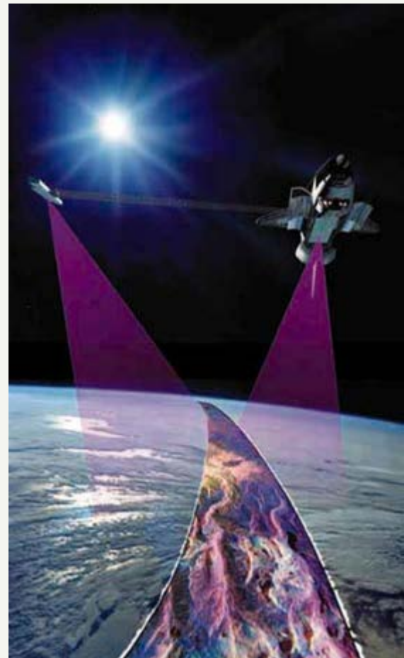
Shuttle Radar Topography Mission C-band interferometric synthetic aperture radar technique, Covers 80% of globe at 30m*30m (Source: Shuttle Radar Topographic Mission (SRTM) Illustration.jpg)
