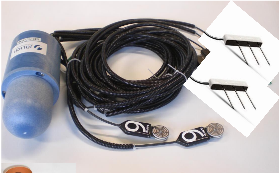
Sensor Unit (GS3 and MPS-6 probes)
